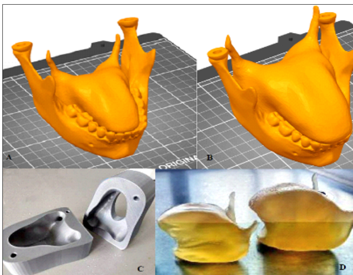
Fig. 2. 3D-printed tongue prototypes with 100% (A) and 125% (B) volumes in the mandibular space, a tongue mold made of PLA (Prusa PLA, Prusa Research a.s., Prag, Czech Republic) (C), and ballistic gel tongue models with 100% and 125% volumes (D) Picture taken by the authors
