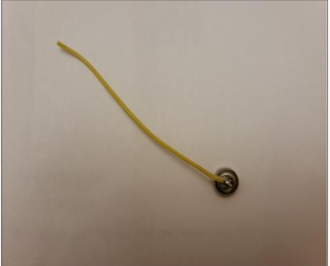
**Fig. 4.** Appearance of the electrode that was used for electrical stimulation.
