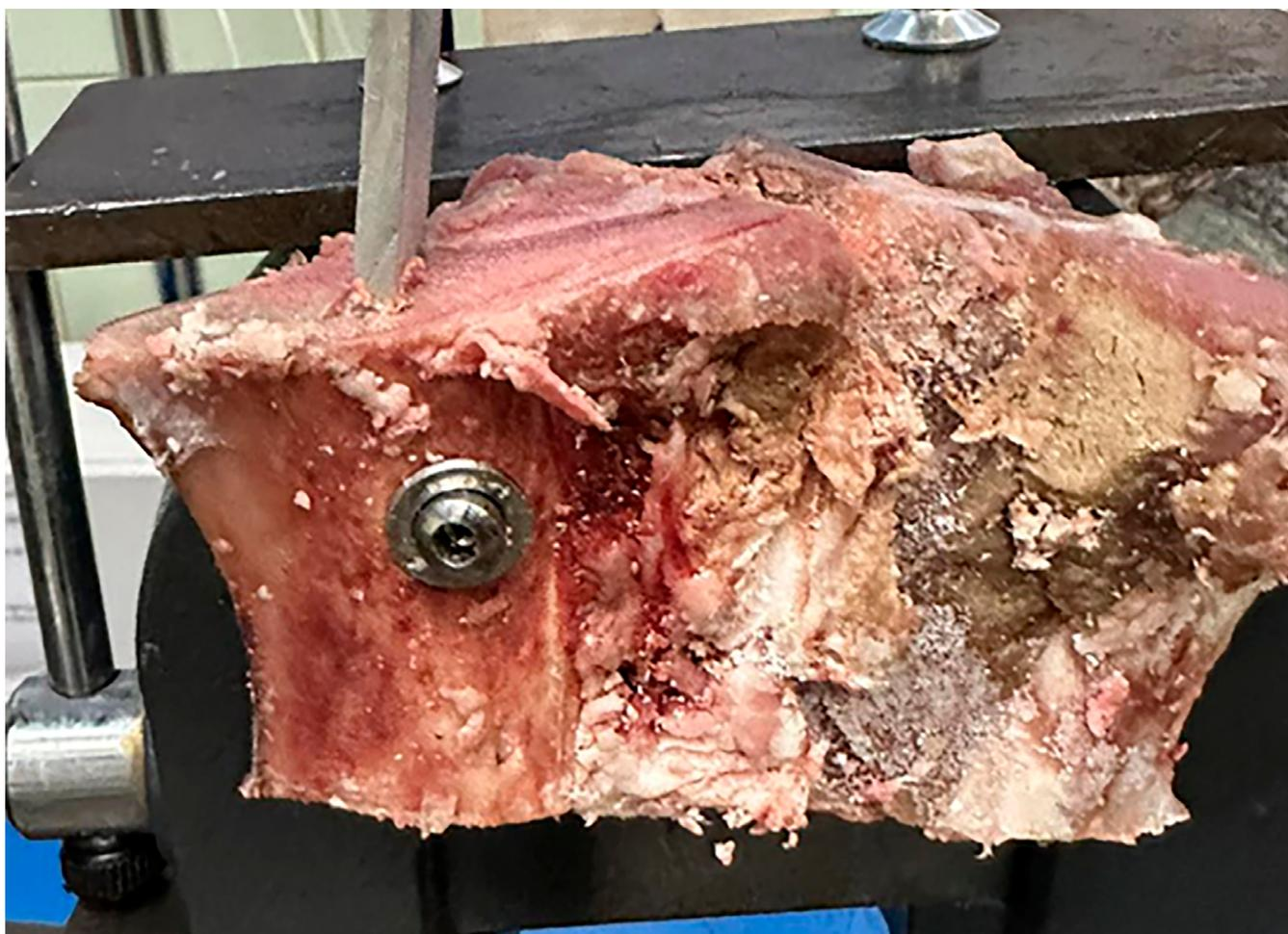
Fig. 7. Secured native specimen of the sacroiliac joint in the research machine.
