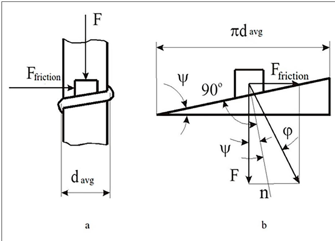
**Fig. 1.** Mechanism of screw interaction with bone. a) – spatial curve of screw-bone interaction; b) – unwinding of one turn along the average thread diameter; F – compression force;  $d_{avg}$  – average thread diameter,  $\psi$  – thread pitch angle,  $n$  – radius perpendicular to the direction of the screw,  $F_{friction}$  – friction force component,  $\phi$  – angle of friction.
