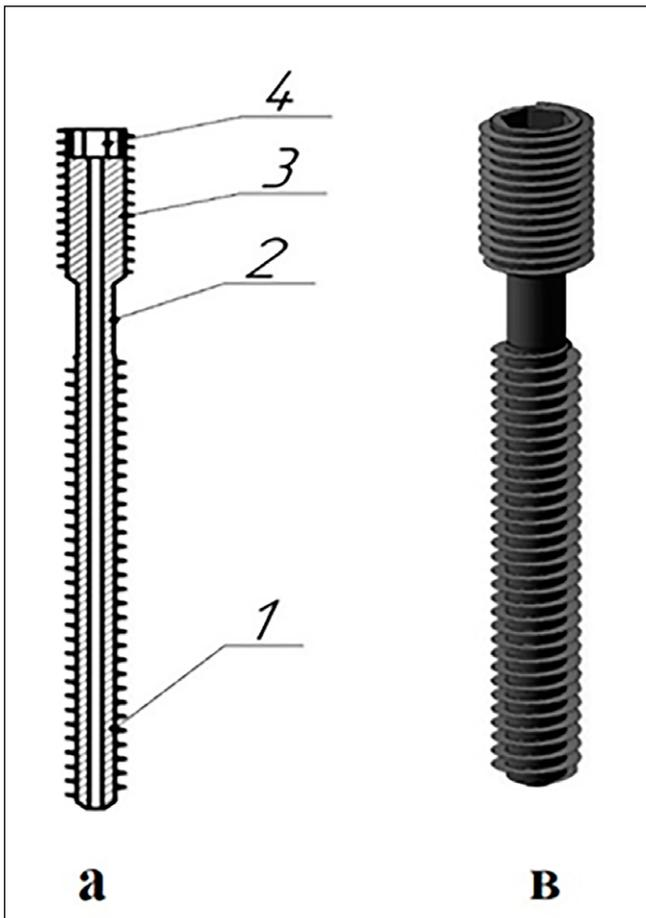
**Fig. 6.** Schematic representation of the counter-compressing screw, where: a) screw drawing (1 – thread with a diameter of 7 mm; 2 – screw body; 3 – thread with a diameter of 9 mm; 4 – hexagonal hole for the key.), b) overall view of the screw (3D model).
