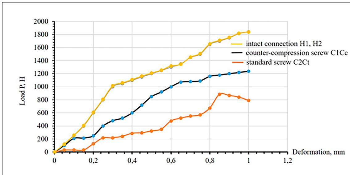
**Fig. 8.** Deformation diagram for cross section deformation of an undamaged sacroiliac joint (H1, H2), damaged joint stabilized with a countersink screw (C1Cc), and damaged joint stabilized with a standard screw (C2Ct).
