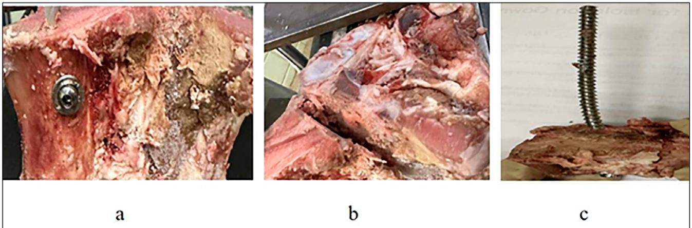
**Fig. 9.** Destruction of the connection, where: a – damaged sacroiliac joint, connected with a standard screw (C2Ct); b – visualized loss of stability under a load exceeding 900N; c – visible deformation of the screw.
