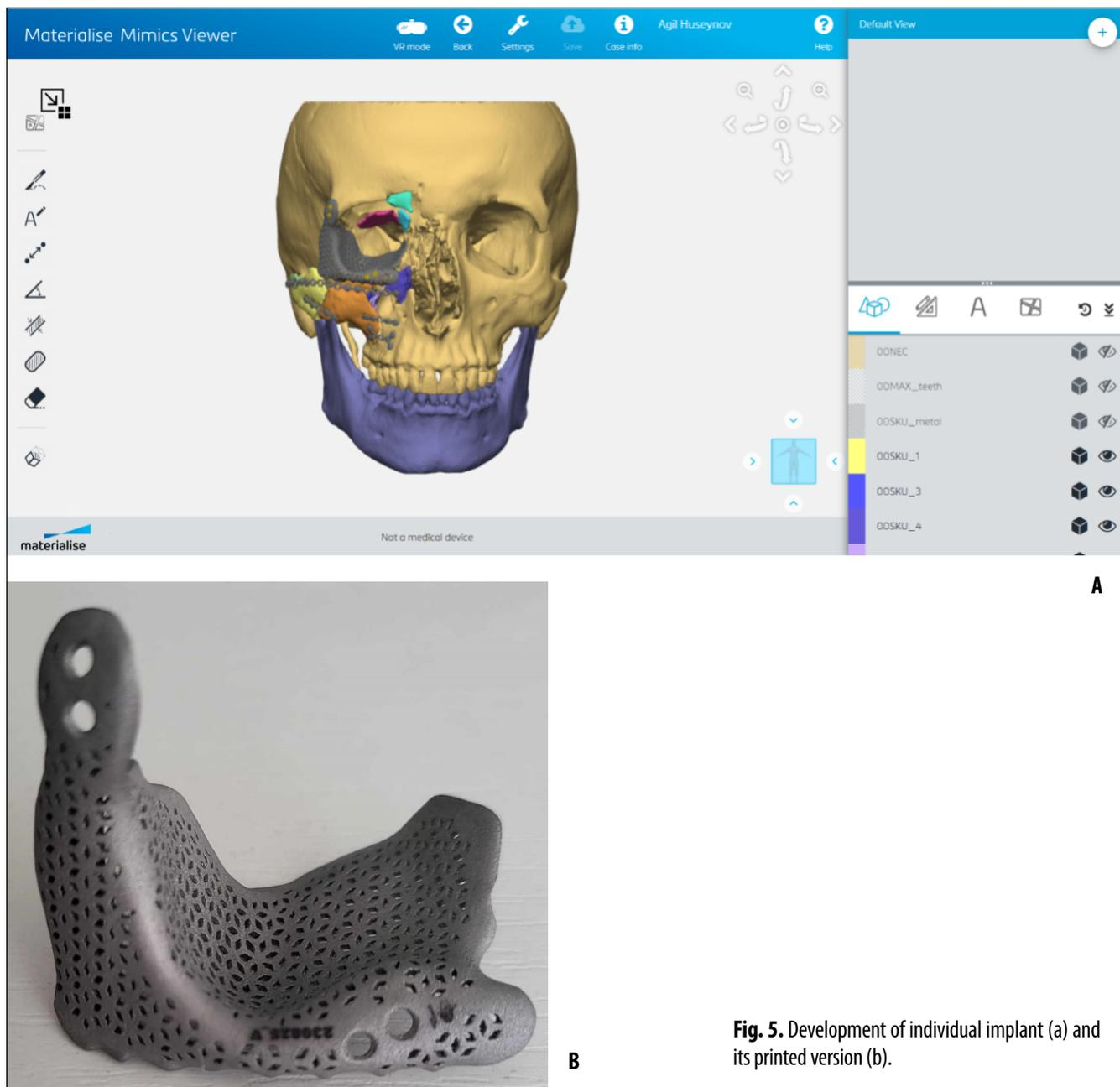
**Fig. 5.** Development of individual implant (a) and its printed version (b).
