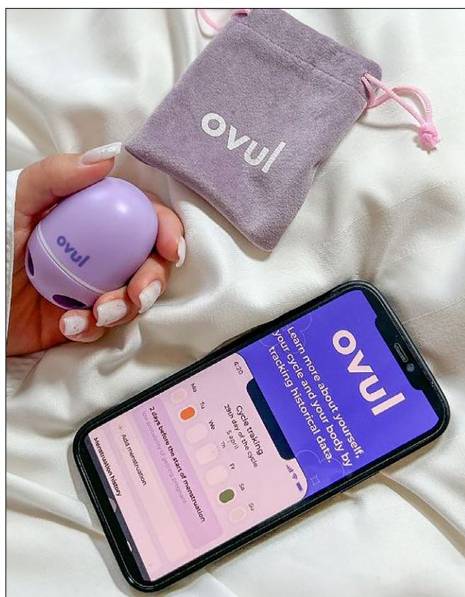
Fig. 3. The Ovul device, which is designed to track ovulation by monitoring the ferning effect in dried saliva samples
